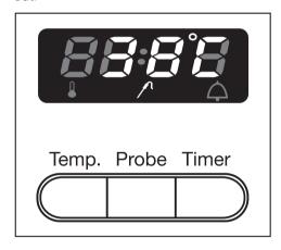
The actual core temperature will appear in the oven display. The lowest temperature that can be displayed is 67°F/20°C, and will not change until the roast probe senses a rise in temperature greater than 67°F/20°C.
